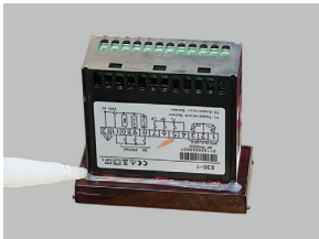
Figure 5: Apply silicone around the frame as shown.
